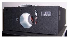
3. Remove the Lens Cavity Front Cover.
